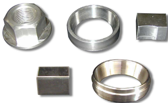
Top Row (Left to Right): Retainer Nut, Lubricity Test Ring, Lubricity Test Block Bottom Row: EP Test Block (Left), EP Test Ring (Right)
