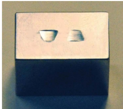
Improperly Positioned Test Block (Note: Two tests may be performed on each face)
