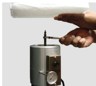
Safe Release of Pressure from a Cell
